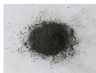
U 3 O 8 Powder Synthesized by calcining UO 2 (NO 3 ) 2 ·6H 2 O
